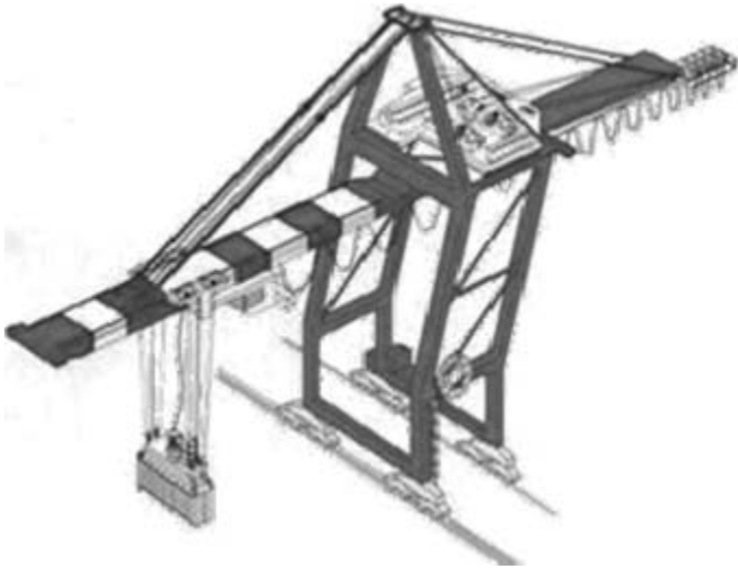
Figure C6.18 Ship-to-shore container crane
