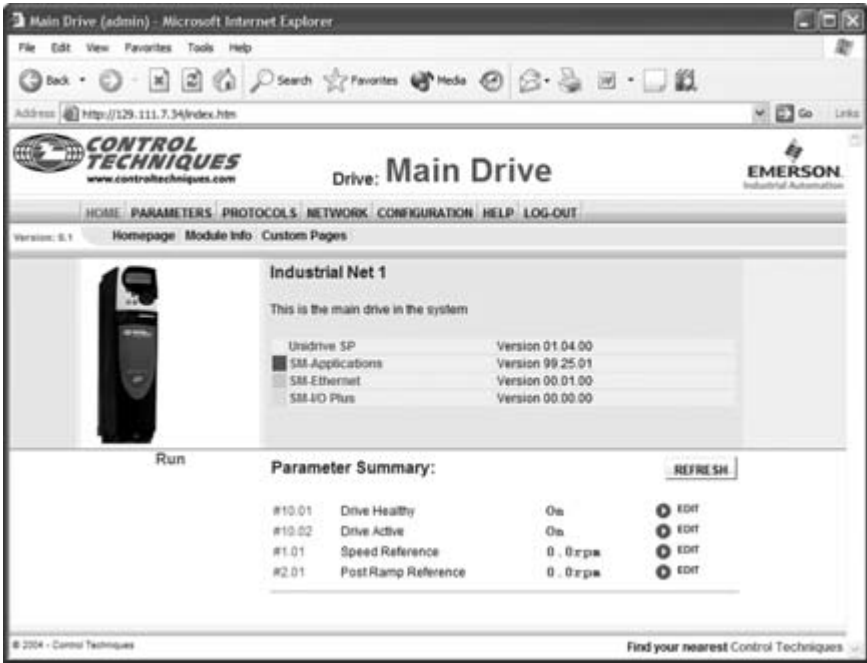
Figure C3.26 A web page embedded in a drive
