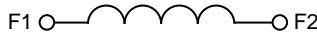
Figure B3.8 D.C. excitation winding of a synchronous machine with two terminals
