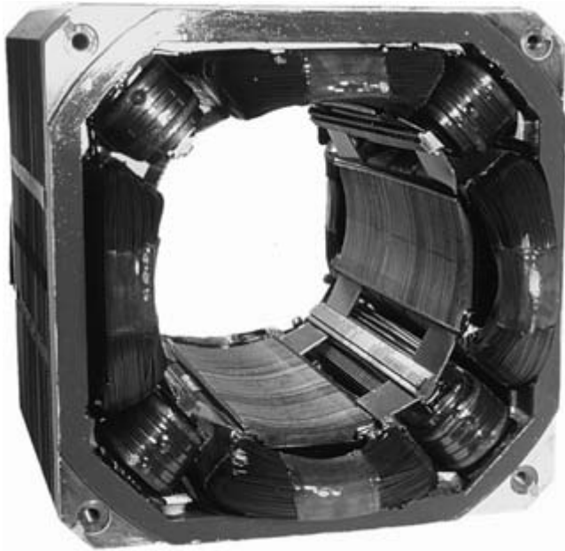
Figure A1.26 A typical four-pole d.c. machine stator (with interpoles) [photograph courtesy of Leroy-Somer]
