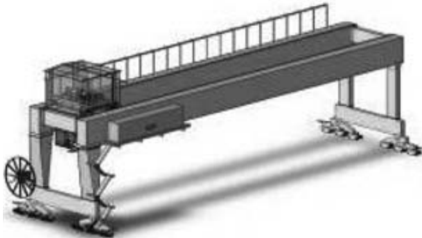
Figure C6.20 Rail-mounted gantry crane
