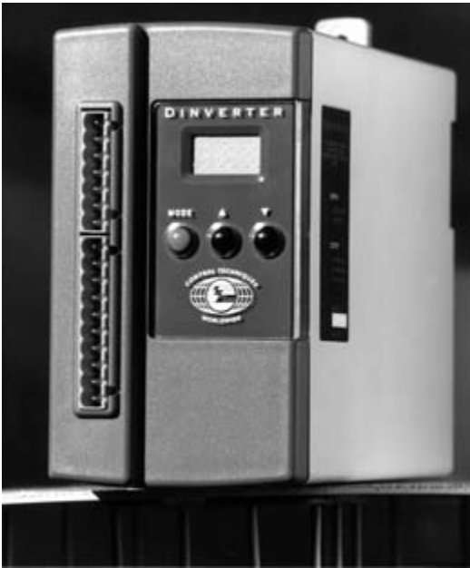
Figure P.9 DIN rail mounting drive with built in EMC filter [photograph courtesy of Control Techniques]
